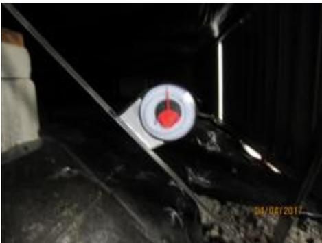
Inexpensive angle gauge to show proper strap angle.
